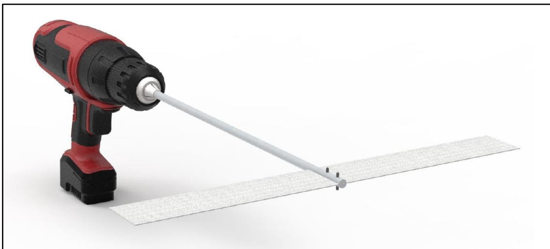
Figuur 7: Cloth and spindle with sawcut
