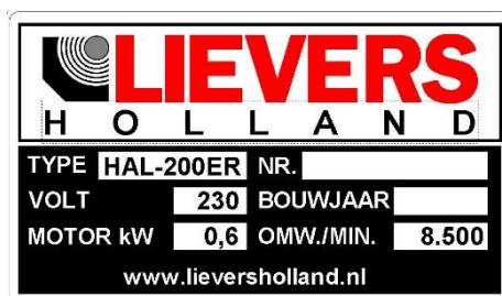
Fig 1: Type plate HAL-200 The type plate can be found on the motor.
